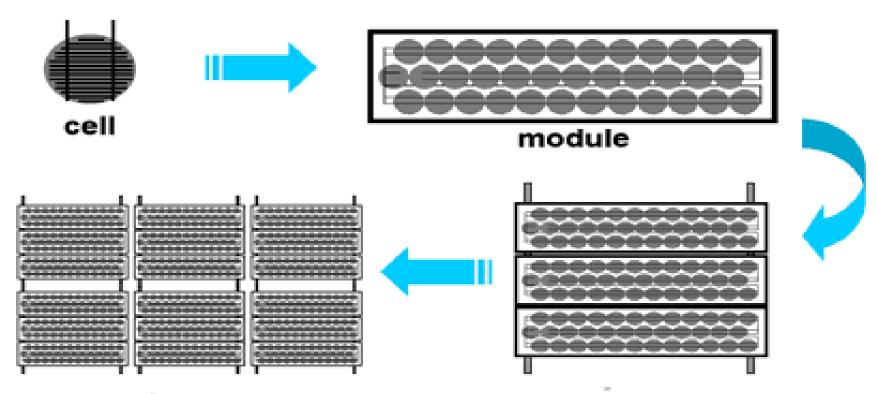
• Photovoltaic cells are connected electrically in series and/or parallel circuits to produce higher voltages, currents and power levels.
